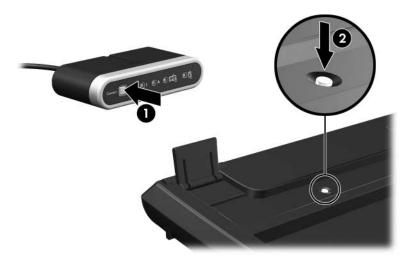
Synchronizing the Wireless Receiver and Wireless Keyboard
